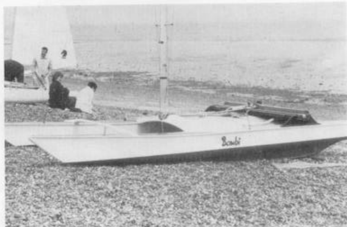
Note Bambi 's solidly-built sliding seat which is limited to athwartship travel making it difficult to trim the boat fore and aft.
