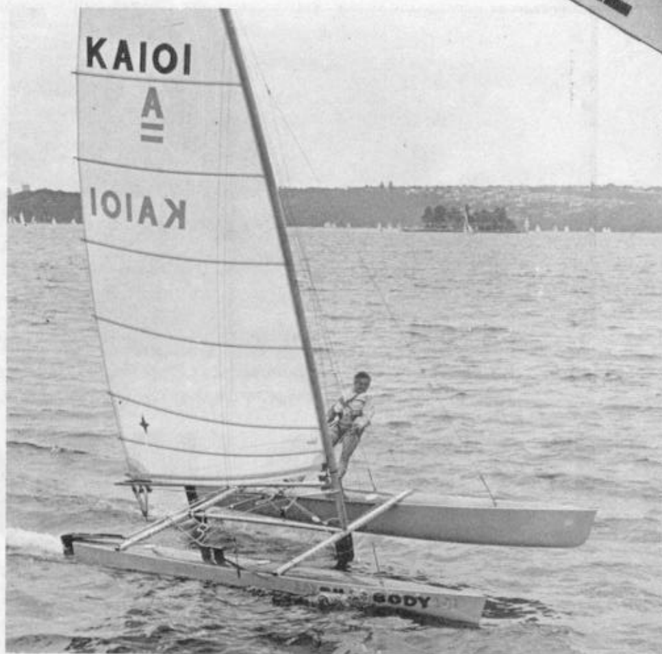
ABOVE: Deep-section hulls have fine entry and exits, move with little fuss. BELOW LEFT: Mainsheet runs on wire hawse across mainbeam. BELOW RIGHT: Mast rotation limiter is simple cleat affair. Line running through daggerboard runs across boat, permits easy raising. Vang leads from wire strop at maststep.
